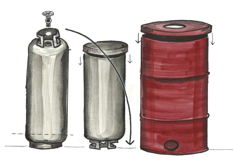
Make two holes at each side of the inferior part of the drum one will be used to light up the wood in the 55-gallon drum and the other one will allow for a better burning. Put on the lid on the drum, in which you will have to make a six-inch diameter hole to induce the stack effect and increase oxygen levels at the bottom. Light up the wood in the bigger drum through one of the inferior holes. You can use the heat generated in the process to cook food on the drum.
